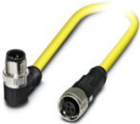
Sensor/Actuator cable, 5-position, PVC, Yellow RAL 1021, Plug angled M12-SPEEDCON, A-coded, on Socket straight M12-SPEEDCON, A-coded, Cable length: 0.5 m
